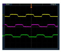
Fig. 12 PWMDAC outputs BemfA, BemfB and BemfC (Vdcbus=160V)
