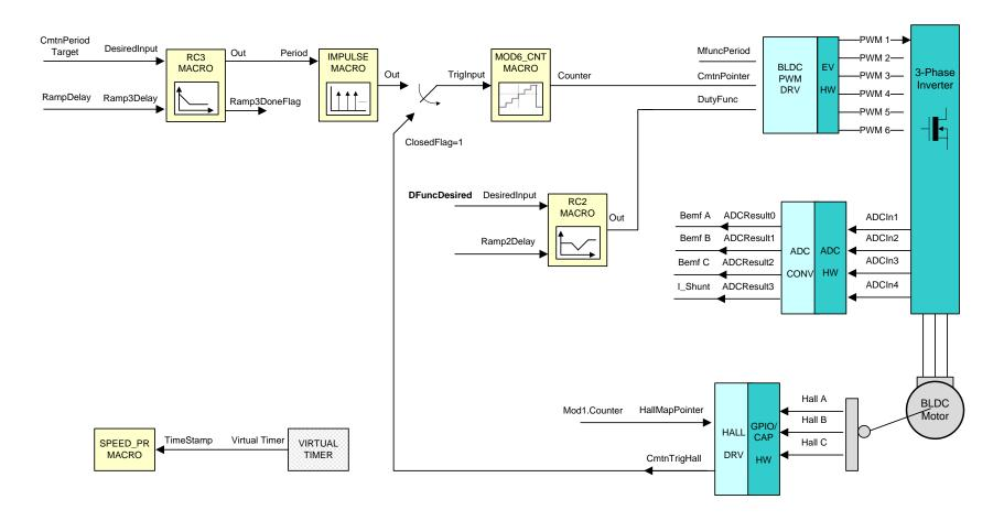
Level 3 describes the closed-loop operation of sensored trapezoidal drive of BLDC motor using Hall sensor.
