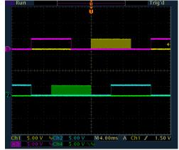
Fig. 10 The PWM outputs , PWM 1 (Yellow) , PWM 2 (Pink) and PWM 5 (Green), PWM 6 (Blue)
