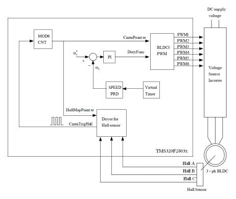
Fig. 7 Overall block diagram of hall-sensor control of BLDC motor
