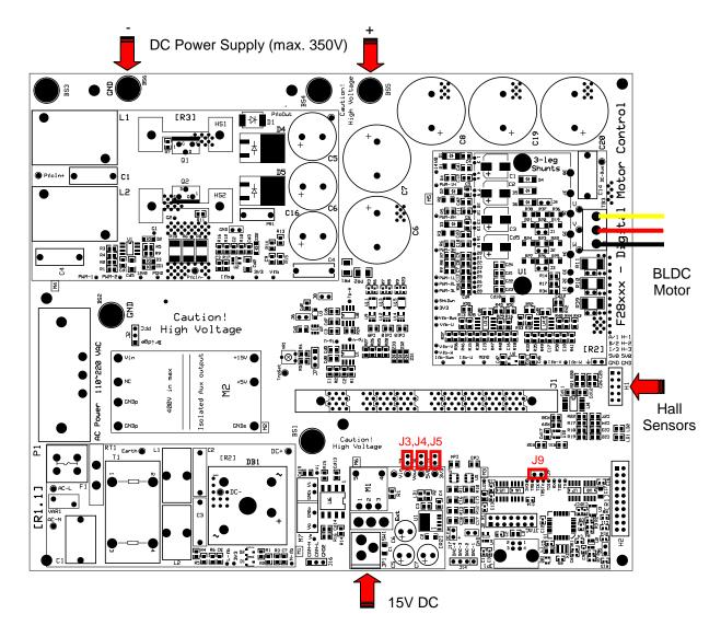
Fig.9 Using External DC power supply to generate DC-Bus for the inverter
