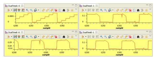
Fig. 14 (a) mod6 counter, (b) BemfA, (c) BemfB and (d)BemfC ( dlog.prescalar=25 and Vdcbus=160V)
