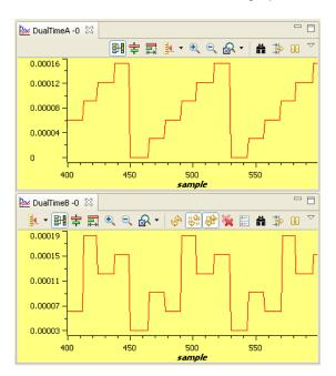
During running this level, the current waveforms in the CCS graphs should appear as follows:
