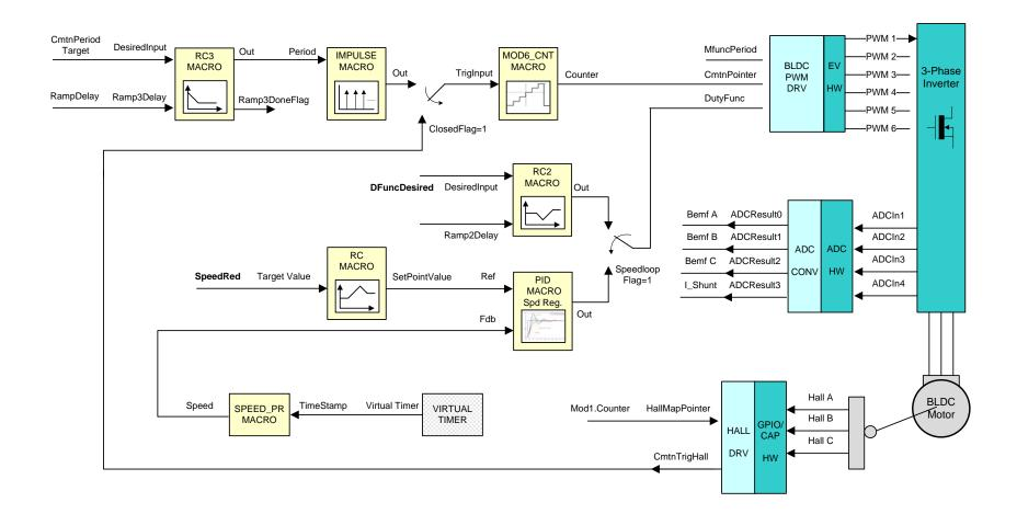
Level 5 Verifies the closed speed loop and speed PI controller.
