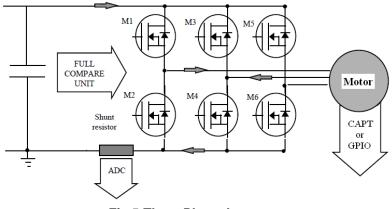
Fig.5 Three Phase Inverter
