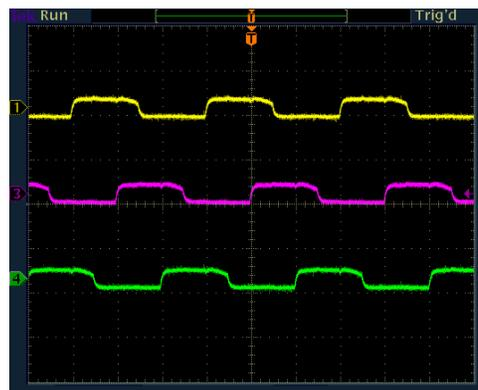
**Fig. 12** PWM DAC outputs BmfA, BmfB and BmfC (Vdcbus=160V)
