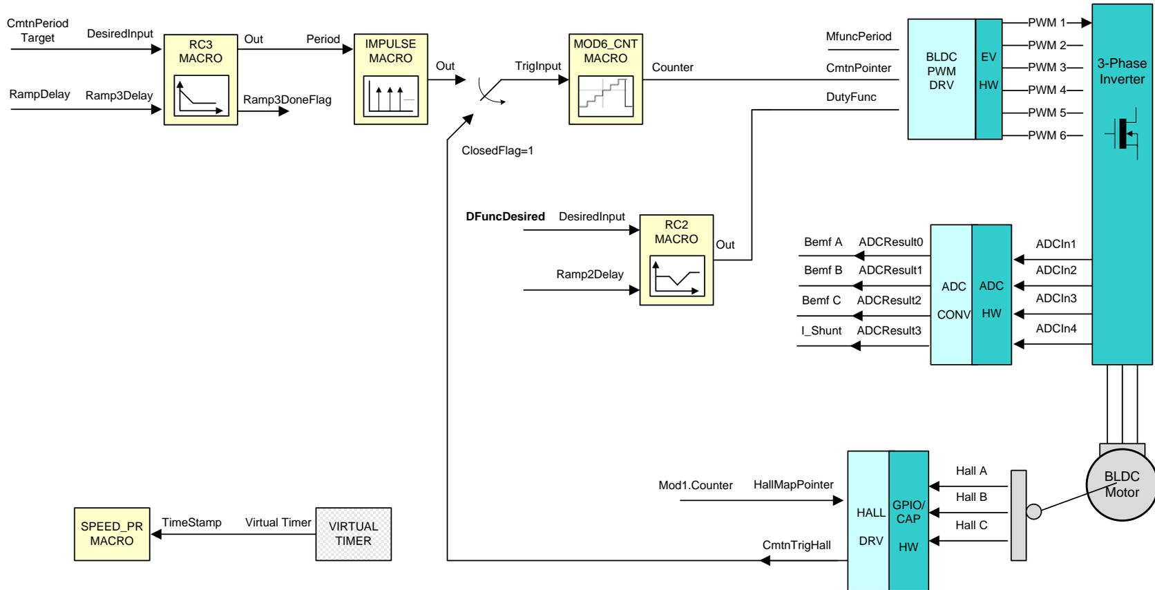
Level 3 describes the closed-loop operation of sensed trapezoidal drive of BLDC motor using Hall sensor.
