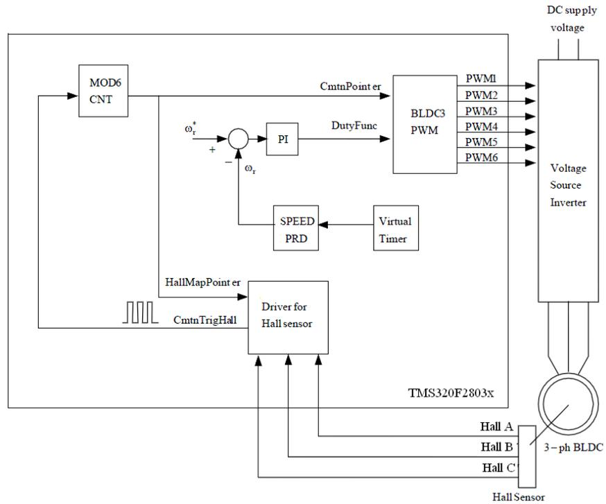
**Fig. 7 Overall block diagram of hall-sensor control of BLDC motor**
