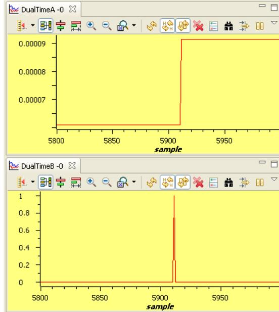
**Fig. 13 (a) mod6 counter (b) impulse output,  $dlog.prescalar=3$**
