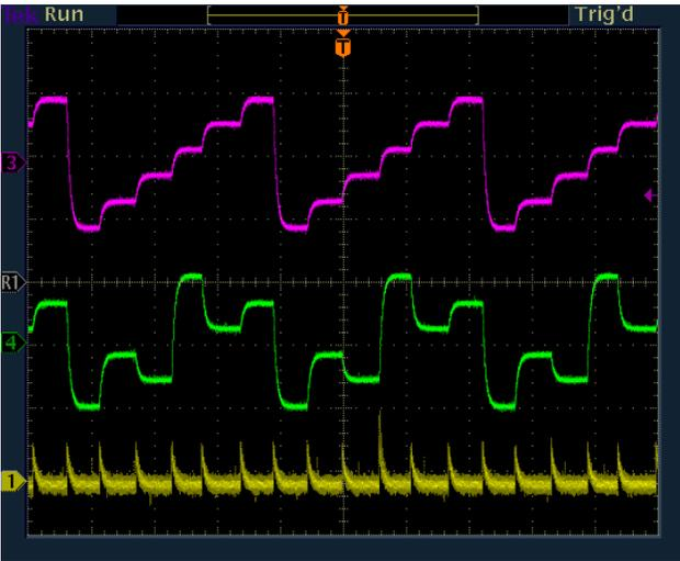
**Fig. 16 (a) mod6 counter, (b) HallGpioAccepted, (c) mod1.trigInput (Vdcbus=160V)**
