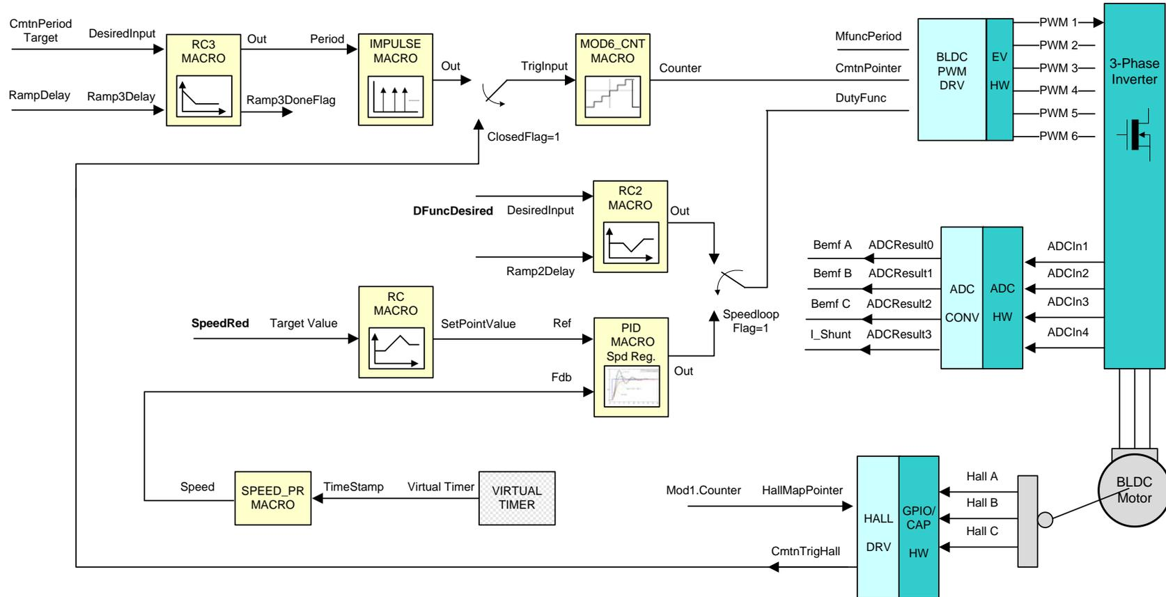
Level 5 Verifies the closed speed loop and speed PI controller.
